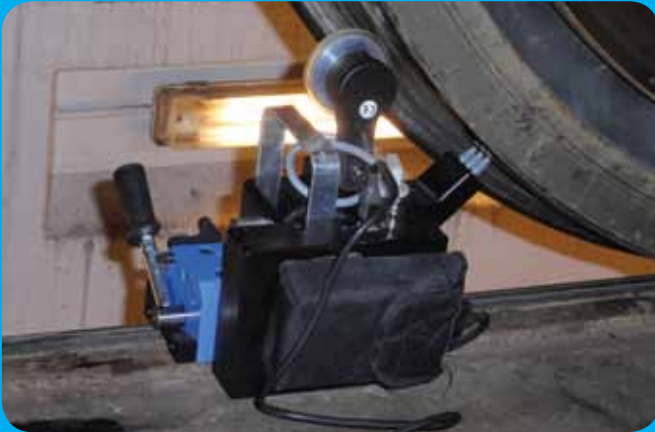
TriTops in two configurations: attached to a rail (left) and to part of an underfloor wheel lathe (right). The instrument takes three measurements simultaneously around the periphery of a wheel. Data are logged to a laptop computer.
