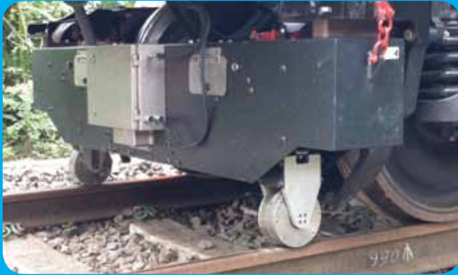
RCA fitted to the bogie of a main-line grinding train.
