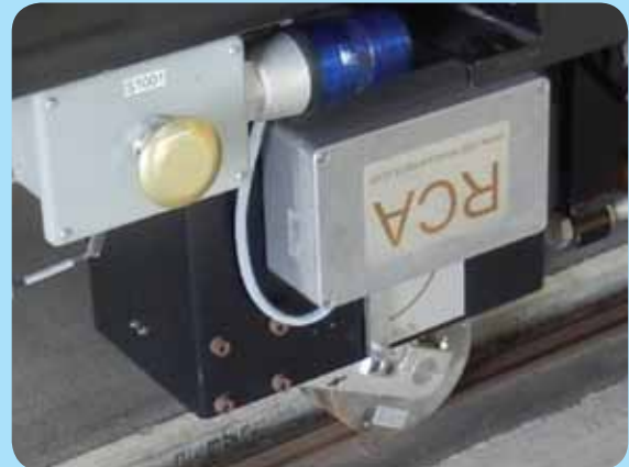
Gauge-adjustable RCA on a small metro grinder.
