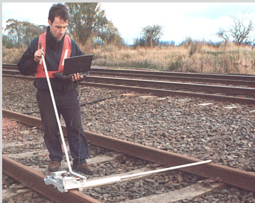
Figure 1: Corrugation Analysis Trolley (CAT) in use
