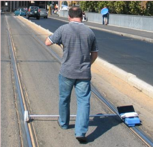
CAT 3 in use on embedded rail: this equipment can be used on heavily worn, deeply embedded rails as well as on conventional Vignole / flat-bottomed rails
