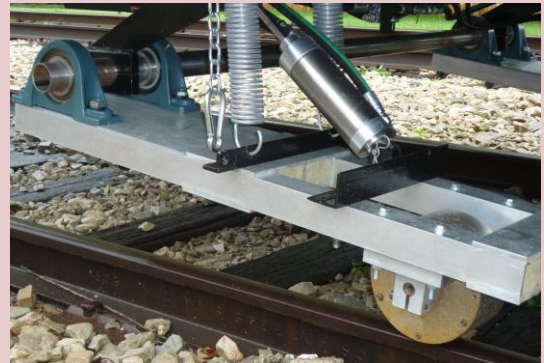
The RCA is usually supplied for routine corrugation measurement on a rail reprofiling train, in particular rail grinders. It has been validated by comparison with a CAT. The equipment can be used during grinding and is sufficiently accurate to show when grinding has been achieved to the requirements of Class 1 of EN13231-3:2006.
