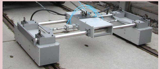
RCA measuring bogie: this equipment is self-contained. It can be attached to a hi-rail or maintenance vehicle, or pushed by hand.
