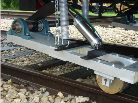
RCA on a metro grinding train, lowered onto rail. Usually the equipment is attached to the vehicle using simple hinged arms, as shown. Alternative arrangements are possible.
