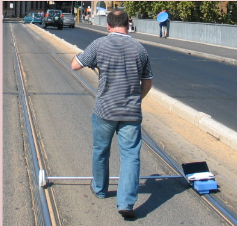
CAT 3 in use on embedded rail: this equipment can be used on heavily worn, deeply embedded rails as well as on conventional Vignole rails
